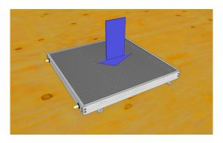
Each panel has to be securely tied down. This is especially true if it is mounted on a rack or on rails so that wind can catch the panels from below. We show a simple set of deck screws here, but depending what method you are planning to use you should follow the directions provided with your mounting hardware. Please remember that these panels are very light so that under no circumstances can you rely on their weight to hold them in place.
