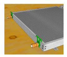
Next the connecting pipes can be pushed into the fittings. The proper insertion depth is close to 3/4". The spacers can be removed **AFTER** the pipes have been pushed in properly.
