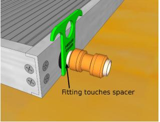
With the spacers in place push two fittings onto the pipes until they touch the spacers. Please note that the fittings will slide onto the pipe with some resistance and it is important to get them well seated.
