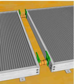
Once completely seated the fittings should be touching the spacers on both sides.
