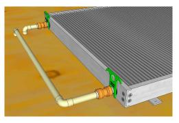
If you are using PEX tubing to connect to the panel array you need to put a plastic insert into the PEX tubing before you push it into the fitting. The plastic insert reinforces the PEX from the inside so that the push-fit fitting can hold on to the tubing securely.
